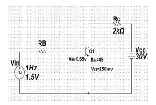
$$V_{in} = I_B R_B + V_{BE} = 0$$
