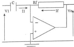
Ex: For the differentiator shown in figure above; if Rf=  $10K\Omega$  and the value of the capacitor is  $0.001\mu F$ , the input signal is given in Fig bellow. Find the output voltage waveform
