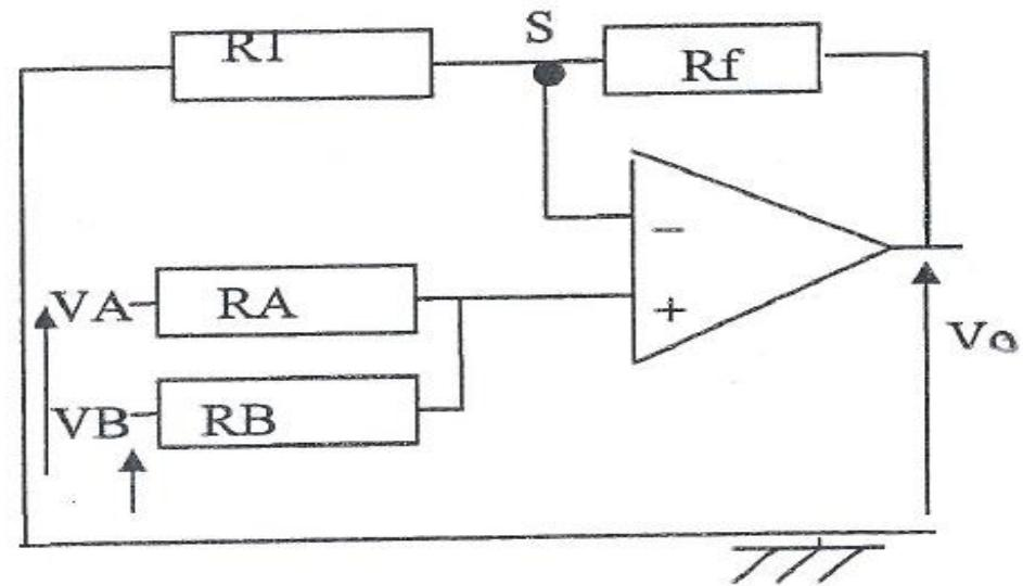
$$V_{in1} = \frac{R_B}{R_A + R_B} V_A \quad (1)$$
